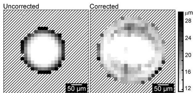
Figure 1: Axial resolution as a function of position in the x,y plane for uncorrected (left) and corrected (right) endoscopic probes (probe length: 1.86 mm; probe diameter: 0.5 mm). The grey scale indicates axial resolution values in microns measured with the technique described in [2].
