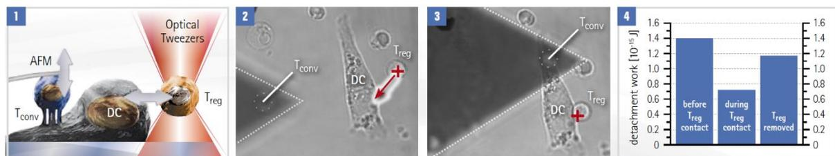
**Figure 1.** (1) Adhesion experiment with dendritic cells (DC) and conventional T-cells ( $T_{conv}$ ). The  $T_{conv}$  is attached to a tipless cantilever, then approached to the surface-bound DC. The cantilever is pulled up and the adhesion forces are measured. A regulatory T-cell ( $T_{reg}$ ) is attached to and removed from the DC with optical tweezers to test its influence on the binding strength.
