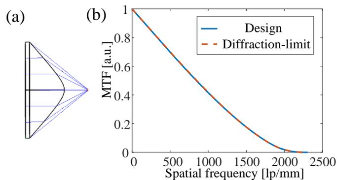
Figure 1: (a) The 0.9 NA microlens design. (b) Modulation transfer function (MTF).
