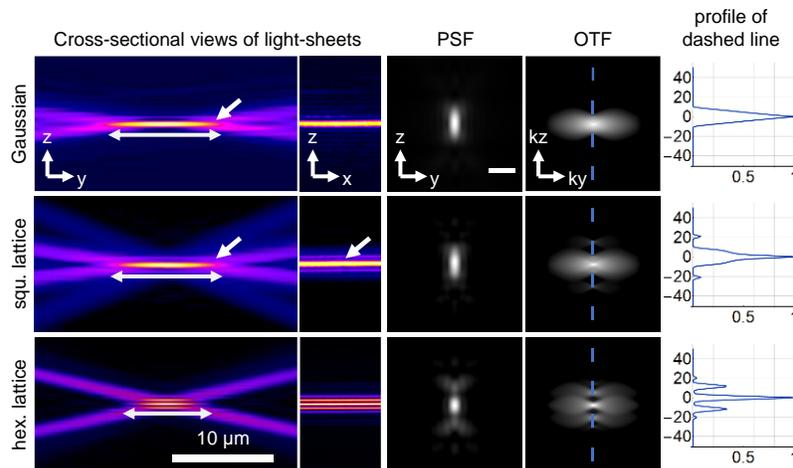
Figure 1: Brief comparison of Gaussian (NA0.24), square lattice (NA0.55,0.44), and hexagonal lattice (NA0.55,0.44) light-sheets. The PSF is generated by multiplying a simulated widefield PSF with the experimentally measured light-sheets. A gamma correction of 0.5 was applied to PSF and OTF images.
