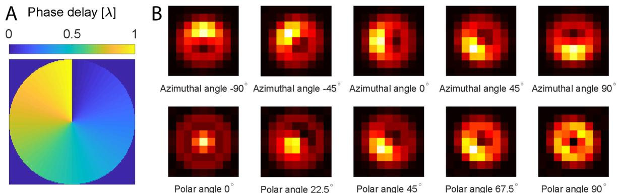
Figure 1: **A)** The phase plate in the Fourier plane applies a  $\pi/2$  phase shift between radially opposing regions. **B)** In-focus PSFs of fixed dipole emitters using the Vortex PSF. Top row has a fixed polar angle of 45 degrees and the azimuthal angle is varied from -90 to 90 degrees. Bottom row has a fixed azimuthal angle of 45 degrees and the polar angle is varied from 0 to 90 degrees. (80 nm pixel size)
