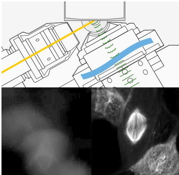
**Figure 1:** sketch of the core optics (top) and imaging without (bottom left) and with aberration correction (bottom right)
