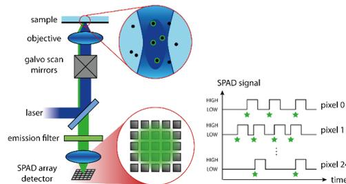
Fig. 1: Imaging the fluorescence signal in a confocal setup with a 5x5 SPAD array detector for FFS analysis.
