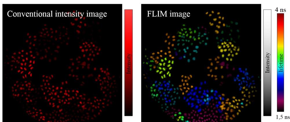
Figure 1. Comparison of a conventional intensity image in red channel and a FLIM image.
