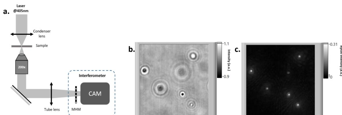
**Figure 1:** (a) Experimental setup of phase imaging microscopy using MHM. (b,c) Image of several particles in solution (200 nm of diameter) by their intensities (b) and by their Rytov approximation intensity after the numerical propagation (c).
