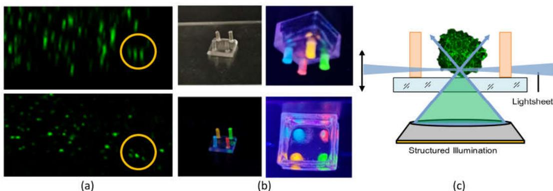
**Fig. 1** (a) 3D printed Quantum Dots, (b) Multiple Material Printing within the XY Plane, samples under Ultra Violet Excitation of 370nm, (c) 3D print on a cover slip.
