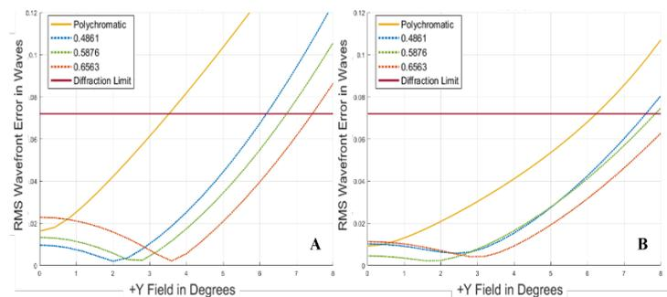
Fig. 1: "RMS v. Field" diagrams of an original tube lens (A) and the optimised tube lens (B). The new cut-off field angle is nearly twice that of the original manually selected system.
