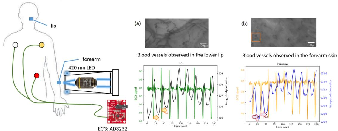
Fig 1. The schematic of micro-angiography. (a) and (b) show the angiography and the temporal evolutions of integrated pixel values in the lip and the forearm versus the ECG signal. The timing differences,  $\Delta t$ , between the integrated pixel values and the ECG indicate pulse wave velocity in the blood vessels, estimated to be 1,200 m/s.
