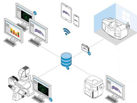
*ZEN Data Storage: Lab setup with multiple acquisition and analysis stations connected by a central data repository*
