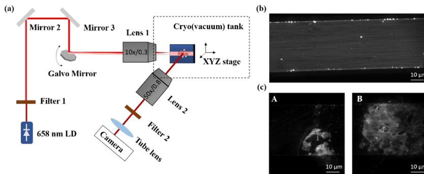
Figure 1: **(a)** Schematic diagram of the chip-based cryogenic TIRF microscopy. **(b)** Near uniform illumination on the waveguide of the chip. **(c)** TIRF images of the plasma membrane of HEK cells at cryogenic temperature.
