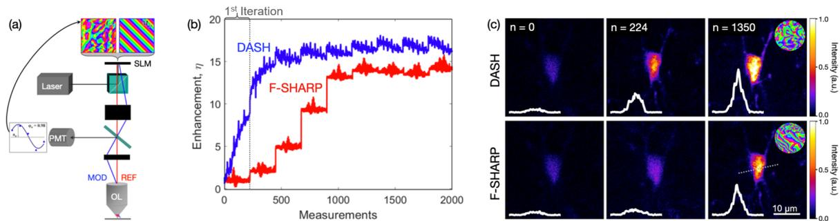
**Fig. 1** (a) Experimental implementation of DASH. (b) Signal enhancement after each mode measurement during DASH (blue) and F-SHARP (red) algorithms. (c) Images of a microglia acquired with no correction ( $n = 0$ ), after the first iteration ( $n = 224$ ), and after convergence of the DASH and F-SHARP algorithms ( $n = 1350$ ), with amplitude profiles along the white, dashed line and the resulting correction masks shown in the inset.
