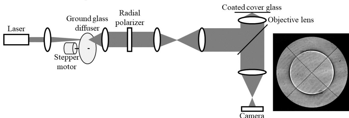
Figure 1: The design of the optical system and a typical BFP image of gold-coated glass
