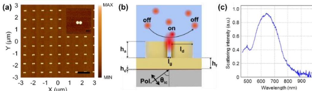
Figure 1: (a) AFM image of gold nanodimer arrays. (b) Schematic field localization by gold nanodimer arrays. (c) Experimentally measured scattering spectrum of gold nanodimer arrays.
