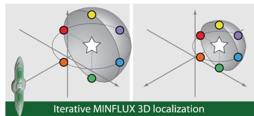
Figure 1: Schematic of the iterative 3D MINFLUX localization scheme using a 3D donut-shaped excitation beam.
