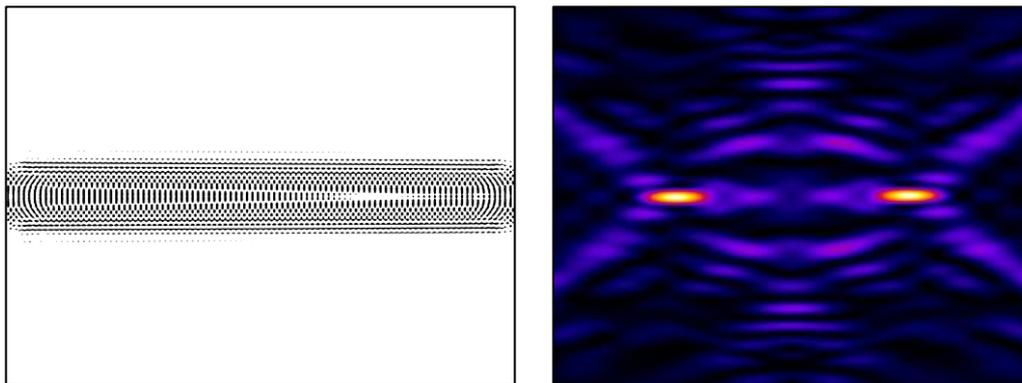
**(Left)** 45-beam lattice pattern, with 80  $\mu\text{m}$  defocus term
