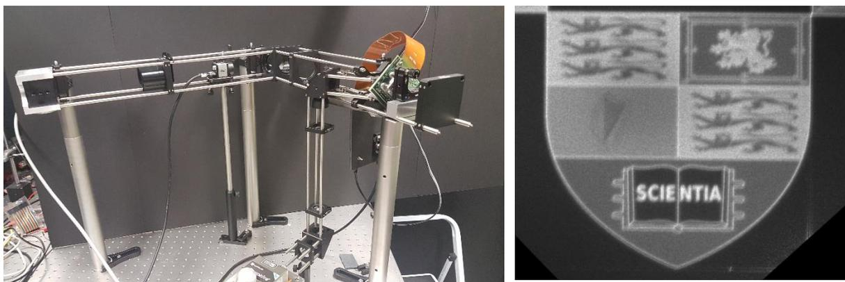
Figure 1 (left): Pattern projection system before it was integrated into the microscope. (Right): Imperial College London crest, created by projecting 100 holograms on the DMD in rapid sequence, and reconstructing the speckle-averaged image using a lens.
