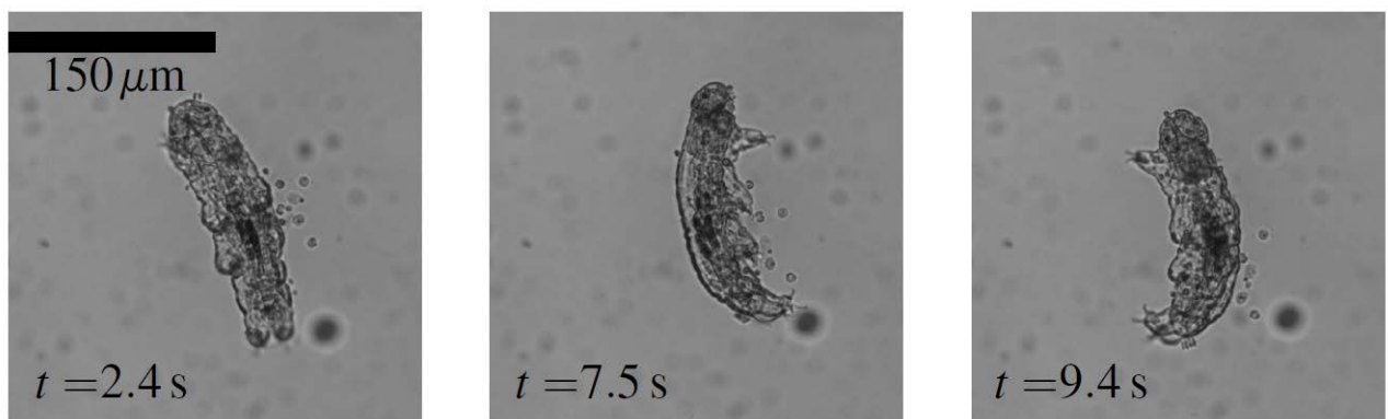
Figure 1: Live tardigrade or 'moss piglet' trapped in 3D in the hybrid acoustic-optical trap.
