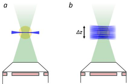
Figure 1: The illumination is confined to a single plane in LSFM (a). Illuminated volume in our setup: the entire depth of field of the detection objective is illuminated and axially modulated
