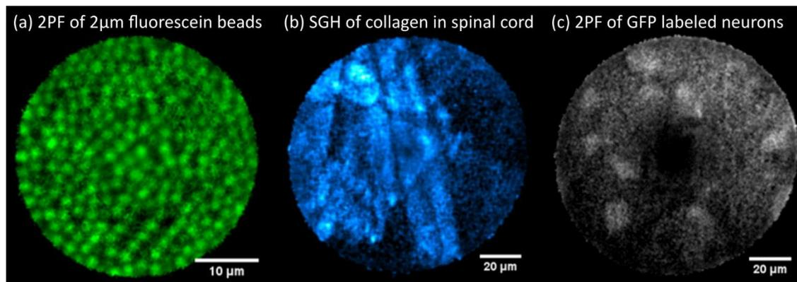
Figure 1: Nonlinear images taken with the endoscope, using our 930nm fiber-based laser.
