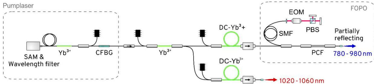
Fig. 1: Setup of the portable fiber optical parametric oscillator. SAM: saturable absorber mirror; Yb<sup>3+</sup>: Ytterbium-doped fiber; CFBG: chirped fiber Bragg grating; DC: double-clad fiber; SMF: single-mode fiber; EOM: electro-optic modulator; PBS: polarizing beam splitter; PCF: photonic crystal fiber
