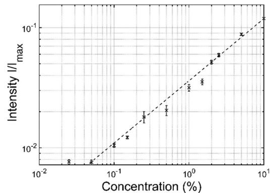
Fig. 2: Dilution measurements:  $I$  is the FM-CARS signal intensity from dDMSO dissolved in water, while  $I_{\text{max}}$  is the signal intensity from a pure dDMSO sample. The detector bandwidth was set to 1 Hz in all measurements.
