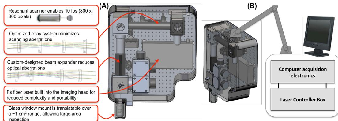
Figure 1. (A) Schematic and overview of the main elements of the scan head. The laser source is built into the scan head, which also contains a laser scanner, relay optics, objective and detectors. (B) Basic layout of the proposed clinical microscope. Sketch is not to scale.
