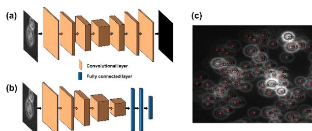
Figure 1. Schematics: (a) FCN for lateral localization and (b) CNN for axial localization. (c) Result of 3D localization of fluorescent beads.
