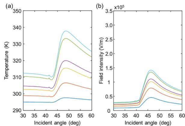
Figure 1 IOTA results: (a) temperature (b) electric field intensity obtained on 50-nm thick gold thin film at  $\lambda = 532$  nm.
