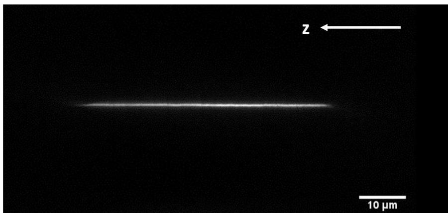
Figure 1: Axial and linear scanning of a laser focus (Numerical Aperture 0.8, 488nm wavelength).
