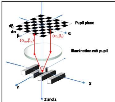
**Figure 1** Illustration of the illumination geometry. The  $(m,n)$  diffraction order of the emerging wave from point  $(\alpha_i, \beta_i)$  is observed at point  $(\alpha_m, \beta_n)$  in the pupil plane
