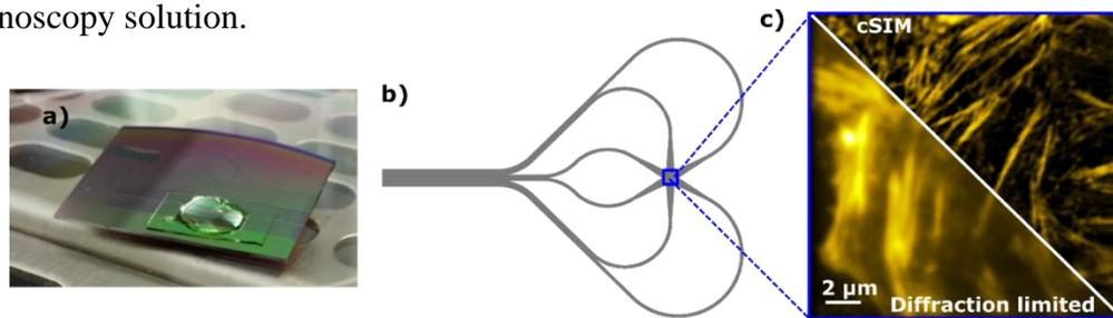
Figure 1: a) A silicon chip is used as the sample substrate and excite fluorescence via evanescent fields. b) By shaping the waveguides in the chip surface, standing wave interference patterns are formed which can be used as the excitation light in SIM. c) Biological specimen is imaged using cSIM showing a clear resolution enhancement
