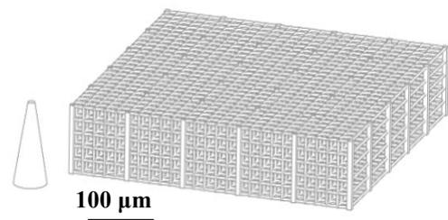
Fig. 1: Representation of a Microatlas micro scaffold.
