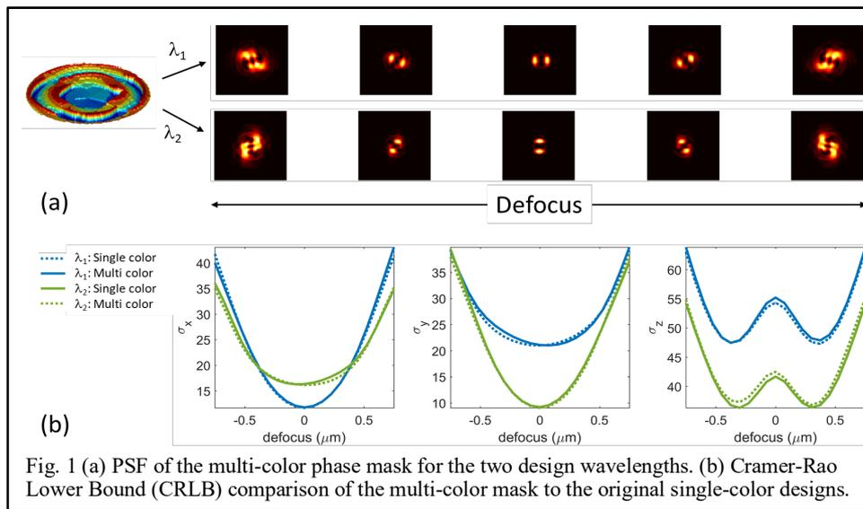
Fig. 1 (a) PSF of the multi-color phase mask for the two design wavelengths. (b) Cramer-Rao Lower Bound (CRLB) comparison of the multi-color mask to the original single-color designs.
