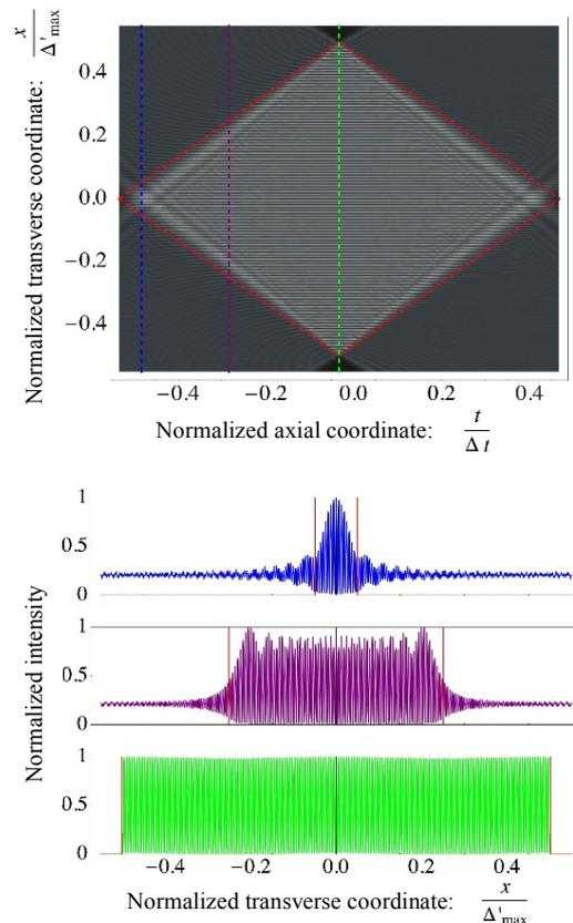
Figure 1: Interference field generated by a WP-based illumination system.
