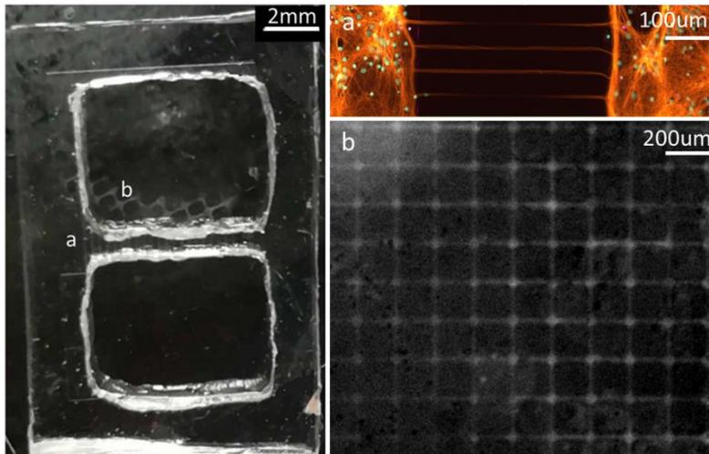
**Figure 1.** A custom-designed microfluidic culture device with (a) two neuronal compartments connected via microchannels. Colin Hockings & Lianne Roode. (b) biofunctionalised proteins for TIRF microscopy.
