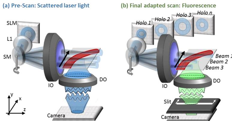
Fig. 1 Setup sketch for a light-sheet microscope using length-adapted Bessel beams.
