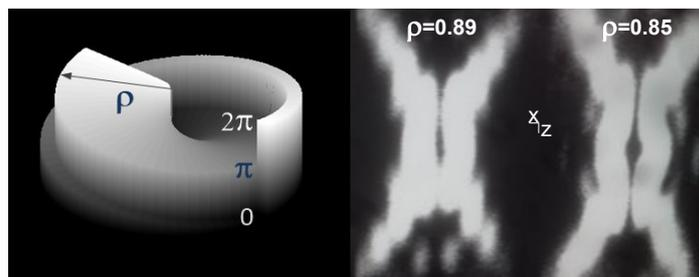
Figure 1: Bi-vortex phase plate and depletion beam axial section at different  $\rho$ .
