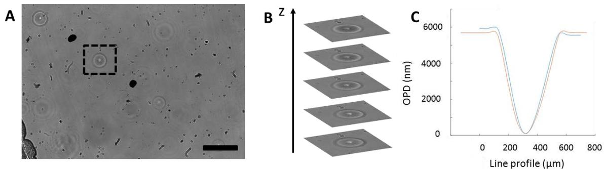
Fig. 1: (A) Full-field of view image of the defects on a glass slide. Scale bar is 1 mm. (B) Z-stack of a cropped region used for numerical reconstruction of the phase map. (C) Reconstructed Optical Path Difference profiles of the cropped region. The proposed set-up (blue line) is compared to the reference method (orange line).
