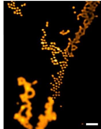
Comparison of a SIM (middle), wide-field (lower left) and filtered wide-field (upper right) fluorescence image of 200 nm TetraSpeck beads. Exposure time per raw frame is 20 ms. Scale bar, 1  $\mu$ m.
