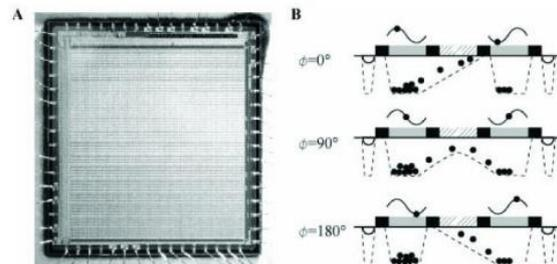
**Fig 1:** The lock-in imager sensor. (A) Microphotography of the sensor. (B) Each pixel has two gates that are controlled with voltages in opposite phase. Thus, the photoelectrons generated in the photosensitive area will accumulate in the two storage areas according to the relative phase of the photon flux and gate potential. Figure from [2].
