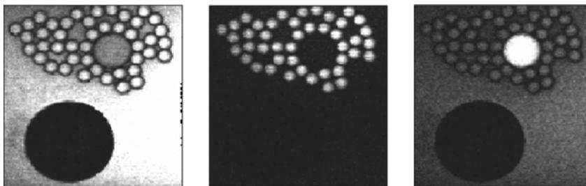
Fig. 1: CRI images of a sample consisting of water, oil and beads of PMMA and PS, each taken with an acquisition time of 125 ms. The energy difference of the excitation pulses was tuned to (a)  $2850\text{ cm}^{-1}$ , highlighting oil, (b)  $2950\text{ cm}^{-1}$ , highlighting PMMA, (c)  $3050\text{ cm}^{-1}$ , highlighting PS.
