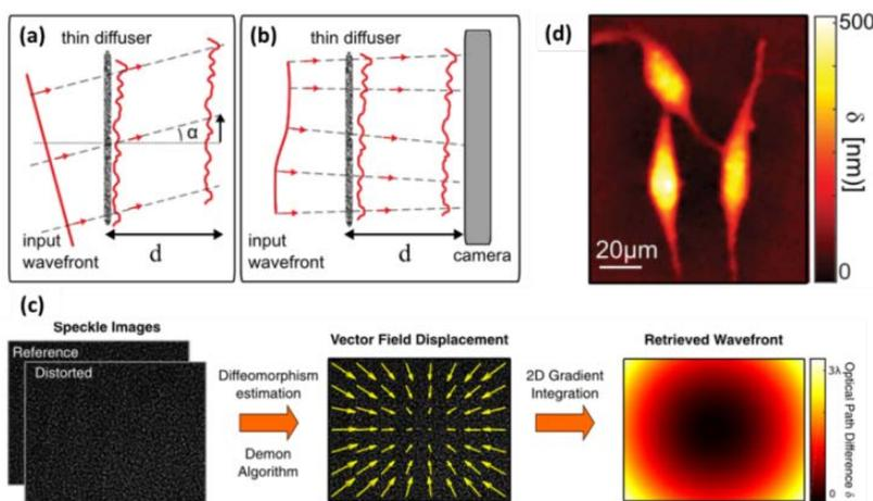
Figure 1: Principle of the thin-diffuser-based wavefront sensor. (a) For a thin diffuser, a tip or tilt angle  $\alpha$  in the impinging wavefront results in a global shift of the speckle pattern by an amount  $\alpha \cdot d$  at a distance  $d$ . (b) For a distorted wavefront, speckle grains are locally shifted. (c) Wavefront reconstruction procedure. (d) Quantitative phase imaging of HeLa cells on a commercial microscope.
