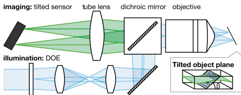
*Novel scanning concept for multi-line 'push broom' scanning. Only two lines are drawn for clarity. By using a tilted sensor, we create a tilted object plane (see inset). A diffractive optical element (DOE) is used to create a multi-line illumination pattern matching the sensor.*
