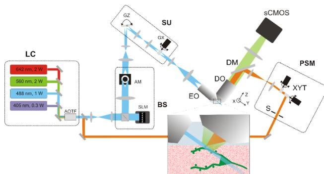
Figure 1: Lattice light-sheet microscope equipped with photostimulation module (PSM) to target any user defined ROI at high spatiotemporal resolution. Inset: Schematic zoom at the sample with light sheet (blue), detected fluorescence (green), and photostimulation beam (orange).
