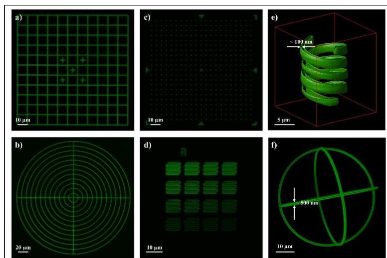
We have developed a new process that enables the etching of long-term stable fluorescent patterns with sub-micrometer sizes in 2D and 3D inside glass (cf. figure on the left). Based on this new process, fluorescent patterns and dedicated image analysis algorithms are shown to be suitable for complete and quick QC of fluorescence microscopes [6]. Non-exhaustively, this new solution
