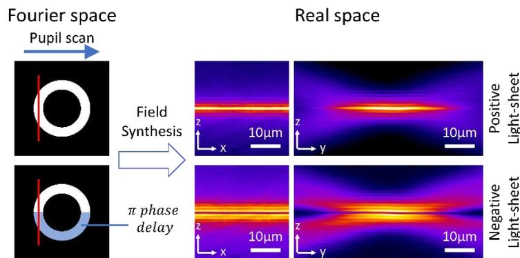
Figure 1: generation of positive and negative light-sheets with Field Synthesis
