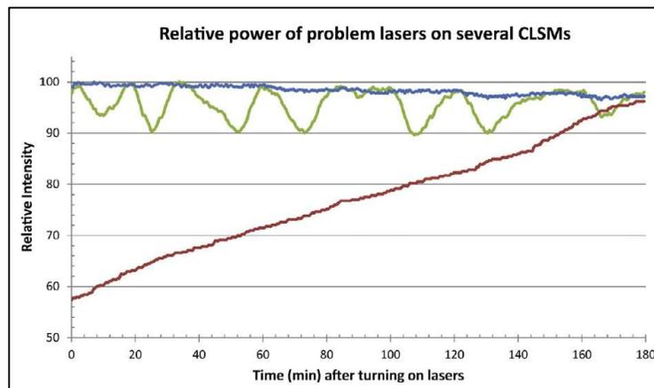
**Figure 2.** Laser fluctuations recorded using power meters on several relatively new confocal microscopes.
