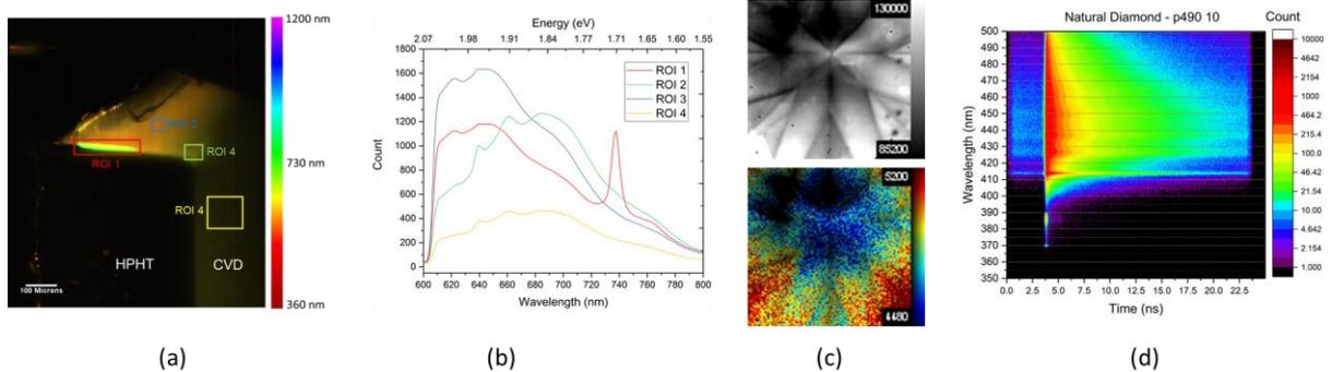
Figure 1 (a) peak wavelength map from hyperspectral data stack and (b) spectra from indicated regions of interest in a hybrid high pressure, high temperature (HPHT) and chemical vapour deposition (CVD) grown diamond with features attributed to  $NV^-$  (ROI 2&4),  $NV^0$  (ROI 3) and  $SiV^-$  (ROI 1) defects; 1(c)(top) shows intensity and (bottom) fluorescence lifetime map of a natural diamond; (d) plot of hyperspectral lifetime data for a single point of interest
