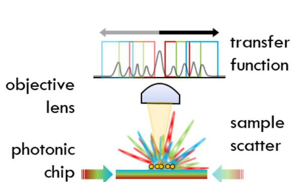
Figure 1: Artificially elongated illumination wavevectors grant access to higher spatial frequency information.
