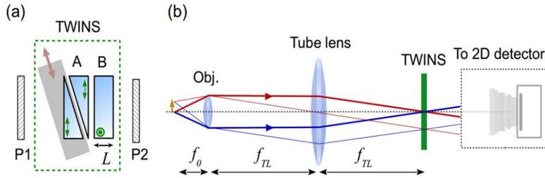
**Figure 1:** (a) Schematic setup of the simplified TWINS interferometer; P1, P2: polarizers at  $\pm 45^\circ$  with respect to the horizontal plane; A-B: birefringent blocks, made of  $\alpha$ -BBO crystal; green double arrow and green circle indicate the orientation of their optical axes;  $L = 2.4$  mm. (b)
