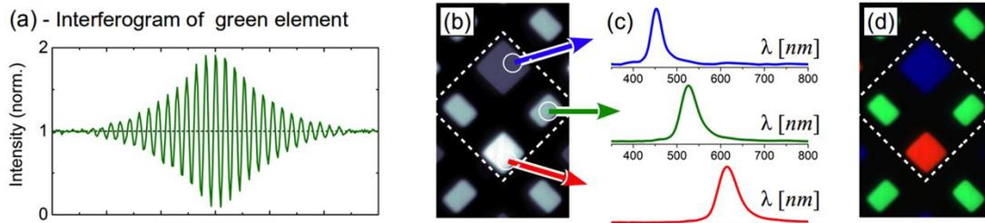
**Figure 2:** (a) Interferogram of a pixel on a green-emitting element of the RGB screen; (b) B/W image of one pixel of the display. (c) Spectra of three points of the image, after FT of the corresponding interferograms. (d) Synthesized RGB picture from the spectral information of each pixel.
