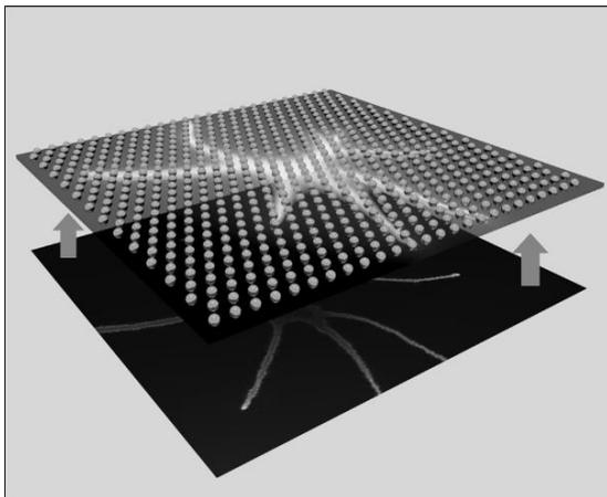
Figure 1: SLM-based projection of an optical pattern calculated to pre-compensate heat diffusion. After photothermal conversion by a gold nanoparticle array, heat diffusion induces the desired 2D temperature repartition.
